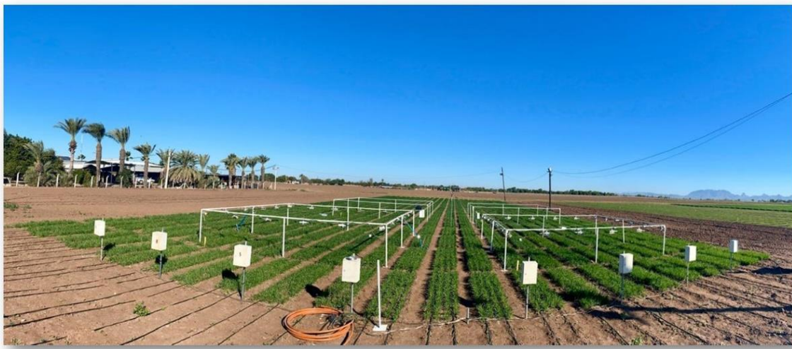
Figure 1. The panoramic image of the field experiment, Yaqui Valley season 2019–2020, comprised four plots, two of which were equipped with heaters and two controls, all connected to a power source that provided heat in the handling plots.
